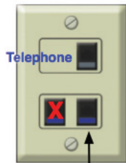
Only the bottom right Ethernet jack is active.
